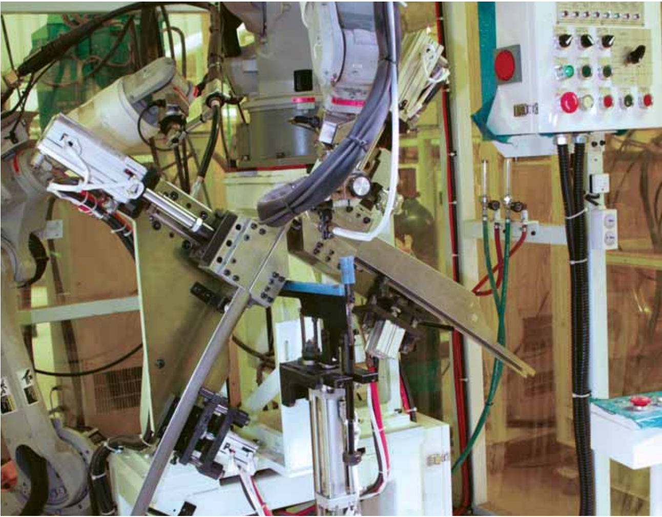
Robotic welding of a car doorframe
